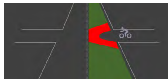
The intersection warning as to be shown on a dashboard
